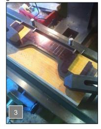
that had already been set square with a DTI. **Photo 3** shows this setup, I used a machined piece of English Oak to clamp the frames to for drilling.
