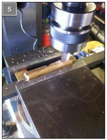
Finishing bogie horns and fitting to frames;
