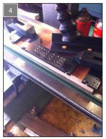
After bolting the frames together, they were turned around reset with DTI and clamped down. (photo 4) All holes were first drilled using a centre drill and followed with the correct size drill. The frames were then turned over for the other side to be countersunk.
